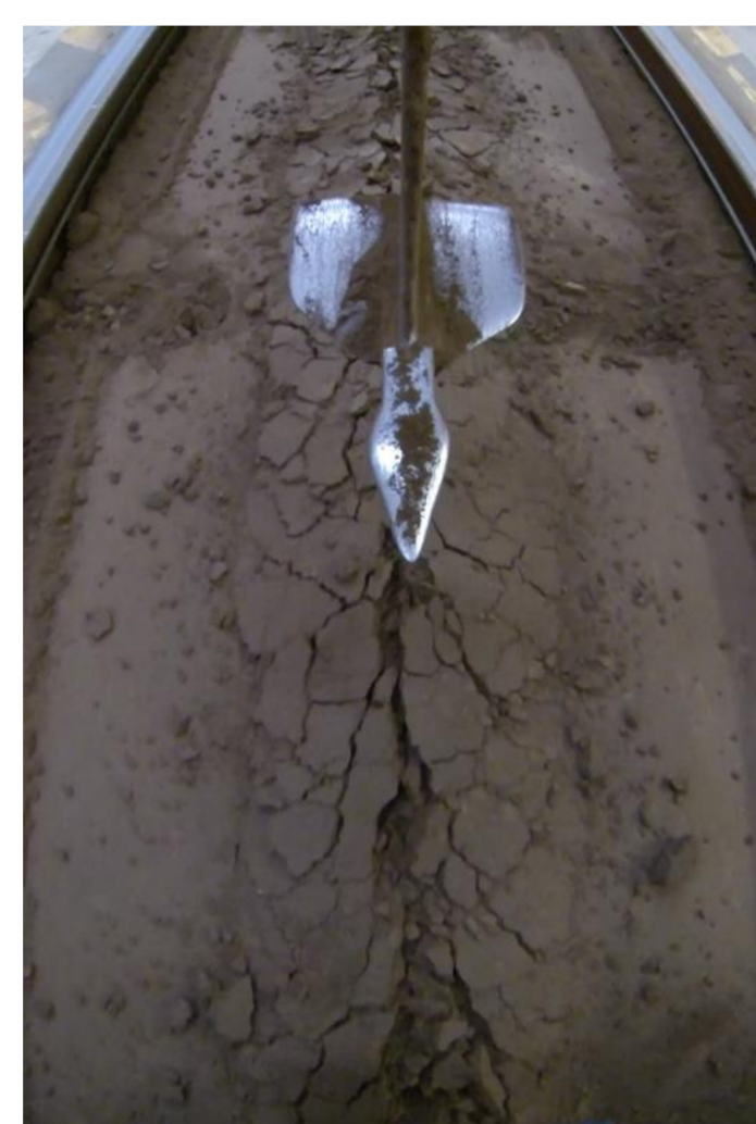
Figure 2: High disturbance subsoiler following an experimental run in Cranfield's Soil Bin
