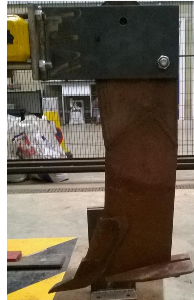
Figure 3: Low disturbance subsoiler mounted in preparation for testing in Soil Bin
