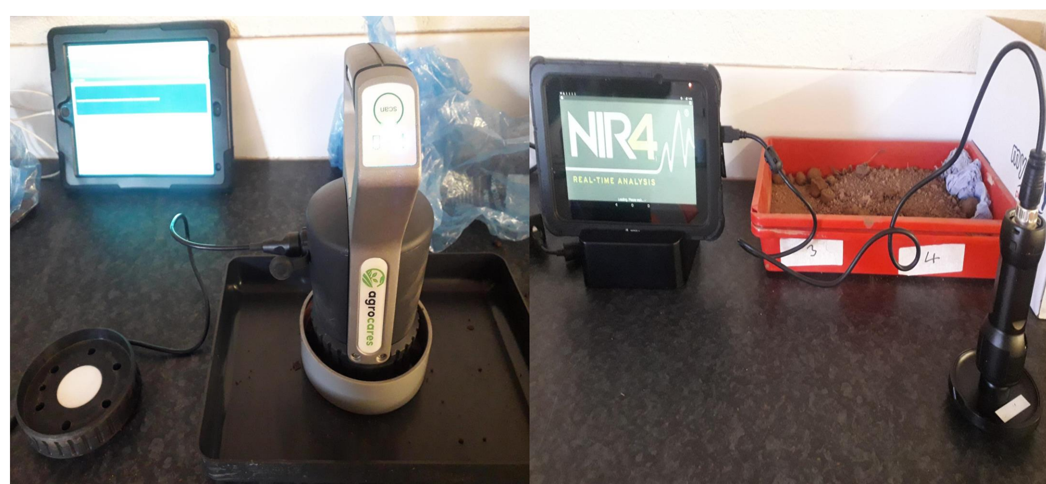
FIG. 2: (a) left: Agrocates soil scanner for soil analysis, and (b) right: NIR4 scanner for forage analysis.
