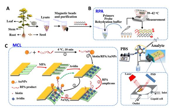
Fig. 3. Schematic illustration of the combined RPA and microcantilever (MCL) assay strategy.
