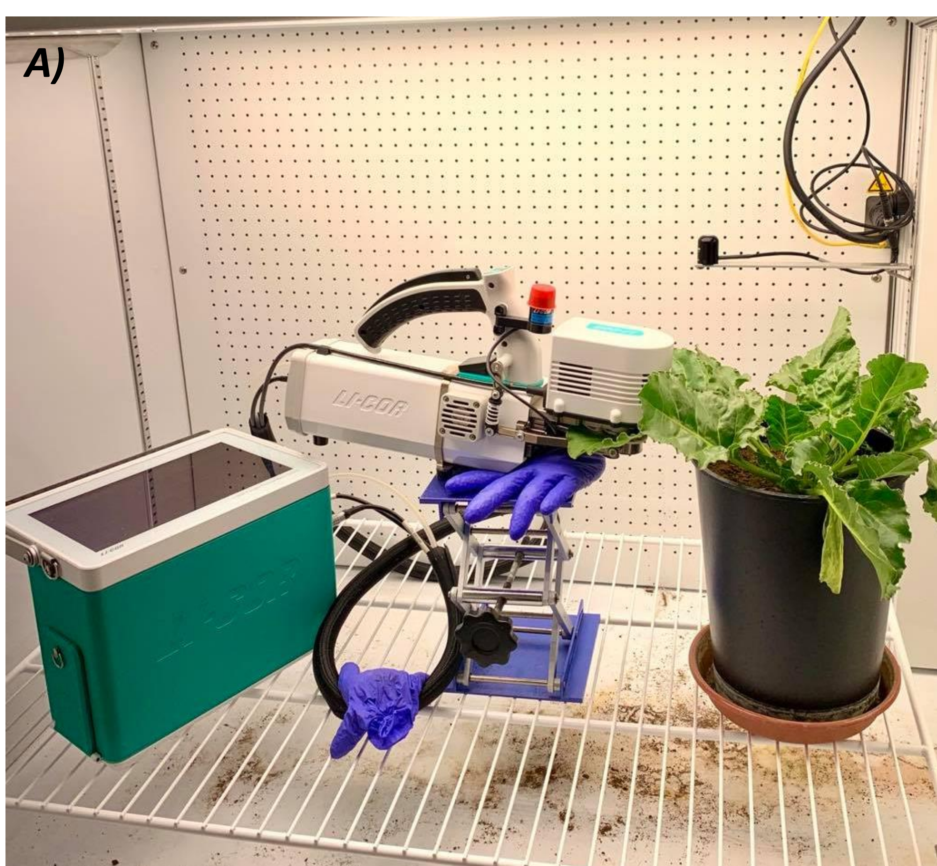
Fig 2. Light response curves to measure canopy photosynthetic potential explained A) LI-COR set up in the growth cabinet. B) Annotated light response curve with parameters measured.
