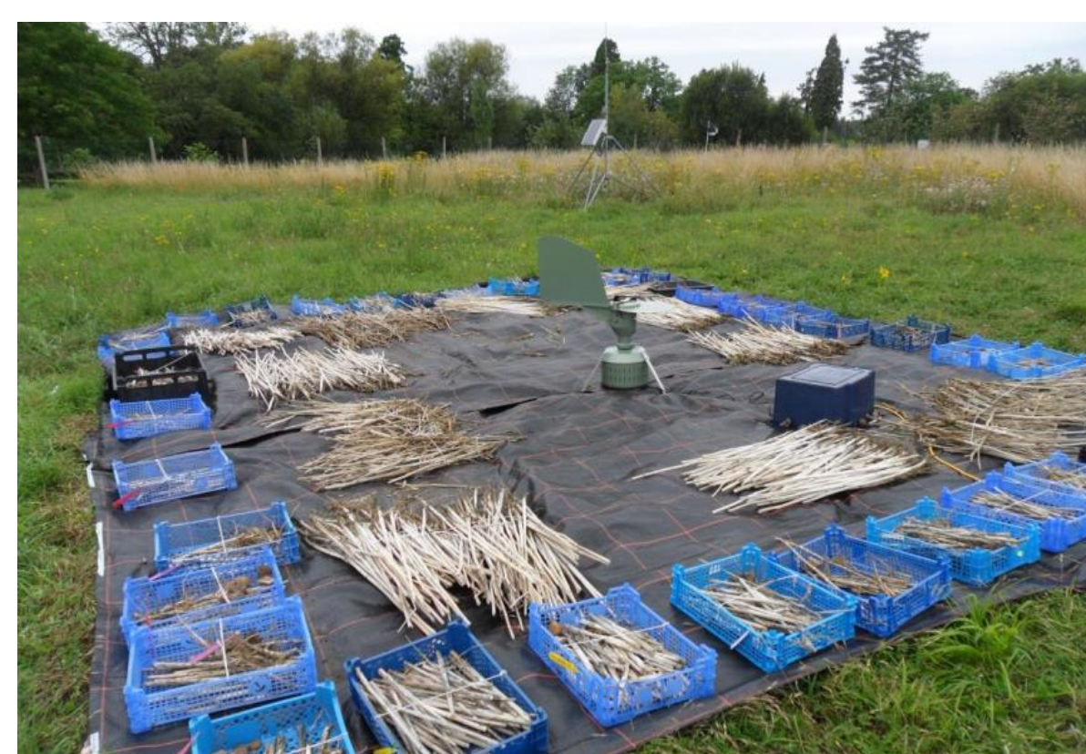
Figure 1: Burkard spore sampler set up at Bayfordbury site in Hertfordshire (2015/16 season). Burkard sampler surrounded by stem debris placed in free-draining plastic trays. Weather station located nearby to collect weather data can be seen in background.
